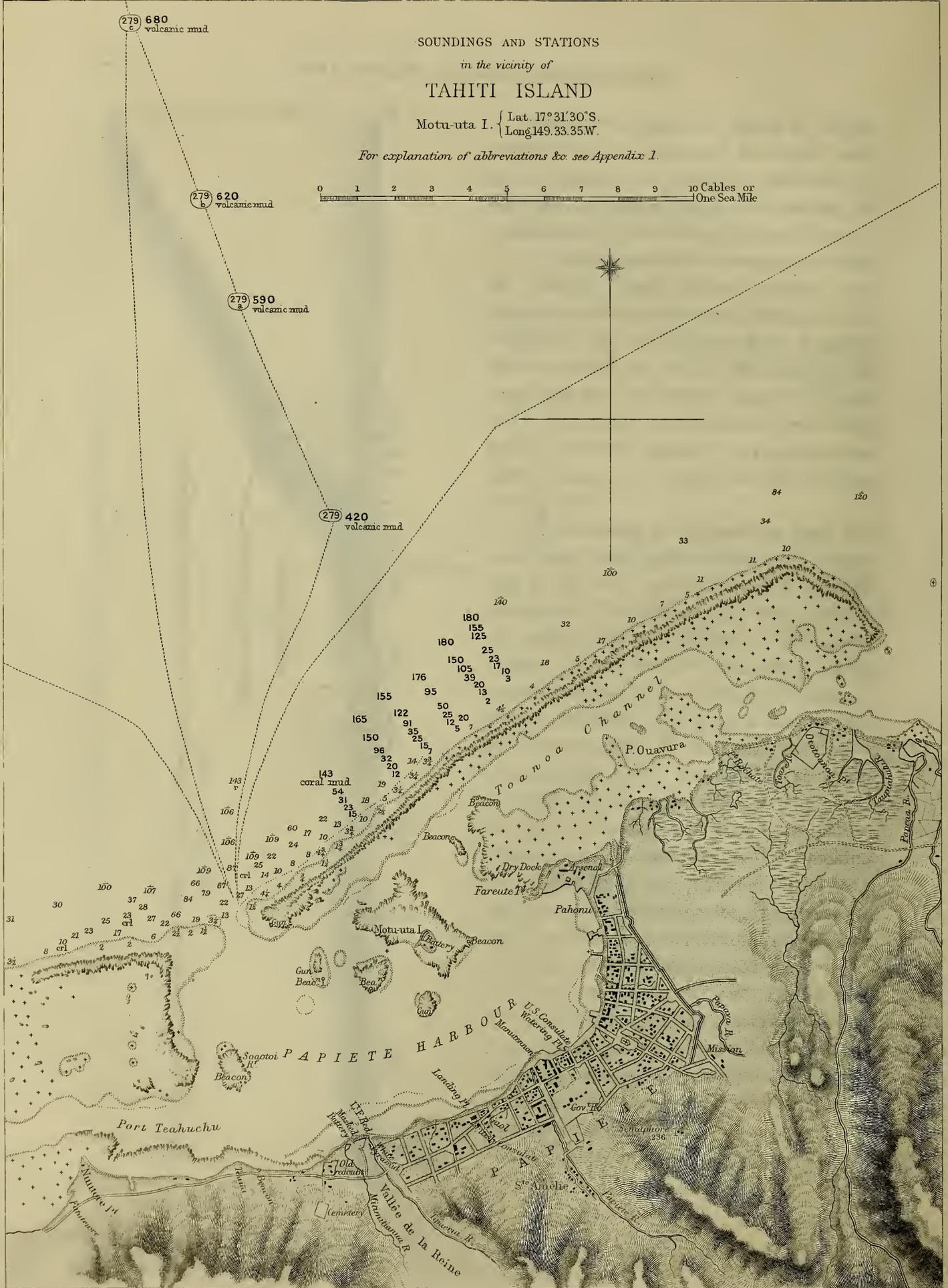
distances apart, previously calculated angles were used, whereas to fix the position of previously agreed upon depths, it became necessary to observe independent angles. In this manner all the lines of soundings were run to such a depth as was possible in a boat, the coast line of the reef was sketched in, and the ship afterwards extended the lines to a distance of 2055 fathoms from the reef."
