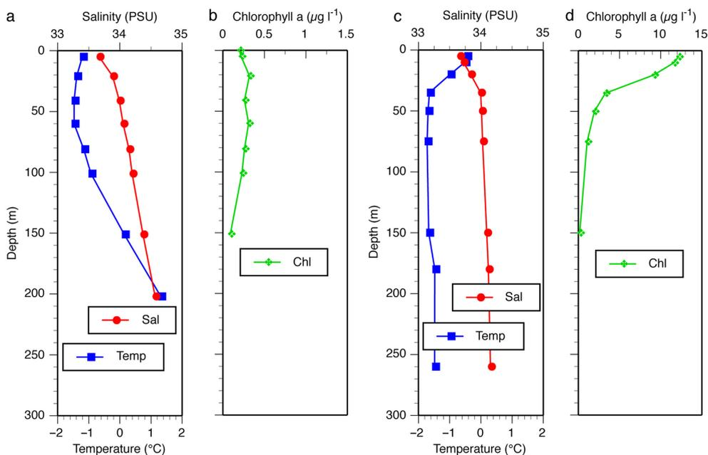
**Fig. 2** Water column profiles of (a, b) station 5, typical of deep off-shore stations, and (c, d) a polynya station, station 18. Note the difference in scales of the chlorophyll profiles. For further details see Tables 1 and 2.
